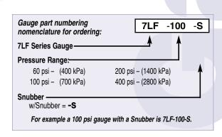
**SPECIFICATION INFO:** Gauge shall be glycerin filled with brass connection with nylon gear, phosphorus bronze Bourdon tube, clear polycarbonate face with a stainless steel cover and EPDM vent plug.
