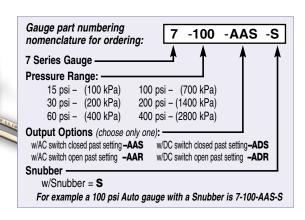
SPECIFICATION INFO: The Automatic Pressure Gauge shall read in pounds per square inch (P.S.I.) and kilopascals (kPa) of pressure and be hermetically sealed from moisture and dirt. Gauge face shall be visible for manual reading and contain an adjustable pressure selector switch. It shall be the Automatic Pressure Gauge as manufactured by The IRROMETER Company of Riverside, California
