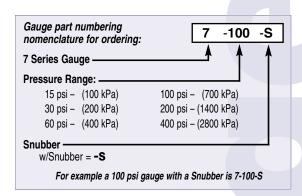
**SPECIFICATION INFO:** Gauge shall have brass connection with nylon gear, phosphorus bronze Bourdon tube, clear butyrate outer face and polycarbonate internal face with a thermo plastic rubber (TPR) cover.
